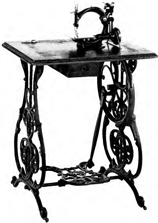
Figure 131.—WILCOX AND GIBBS SEWING MACHINE, serial number 296572, of about 1878. From 1857 to the turn of the century, the style of the Willcox and Gibbs sewing machine changed very little (fig. 39). It was the most popular and the most reliable of the many chainstitch machines. In addition to the basic mechanical patents, Gibbs also patented the design of the sewing-machine head in 1860. In the specifications, he described it as an open ring set on a base or pedestal. The lower part of the open section supported the cloth plate. The design of the head, intentionally or not, formed a perfect letter G, the initial of the inventor. Later the machine head as a letter G was incorporated into the company's trademark. Additional patents were also granted to James Willcox for a leg and treadle design and to Charles Willcox for mechanical improvements.
